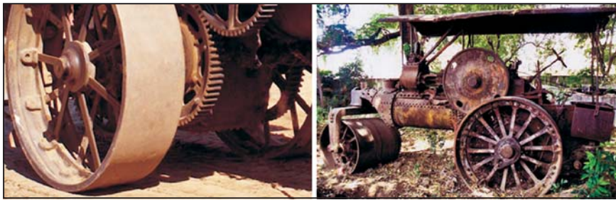
Ratchet wheel fixed to the back wheel of steam road roller (Left) Steam Road Roller's picture published in Hindu Daily (Right)
